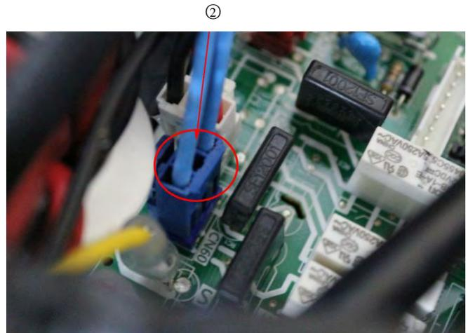
3) Pull out connectors of the condenser coil temp. sensor(T3), outdoor ambient temp. sensor(T4) and discharge temp. sensor(T5).
