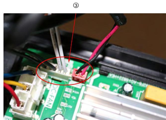
4) disconnect the electronic expansion valve wire
