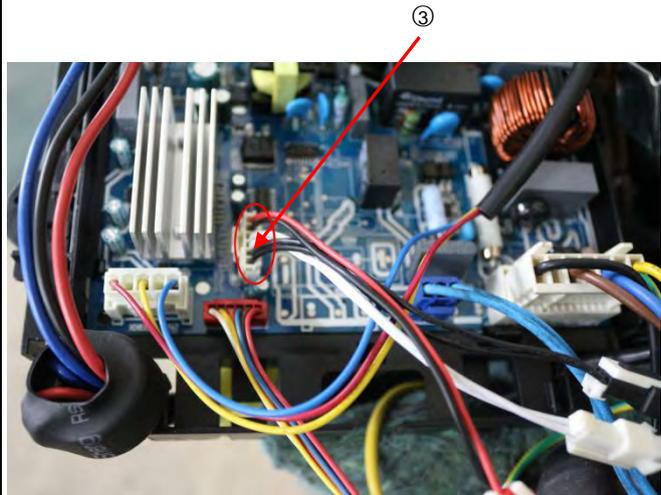
4) disconnect the electronic expansion valve wire
