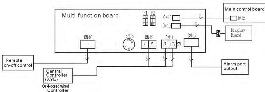
Note: It must use shield cables to connect with 4-cored wired controller and Central controller. The length should not exceed 50m.
