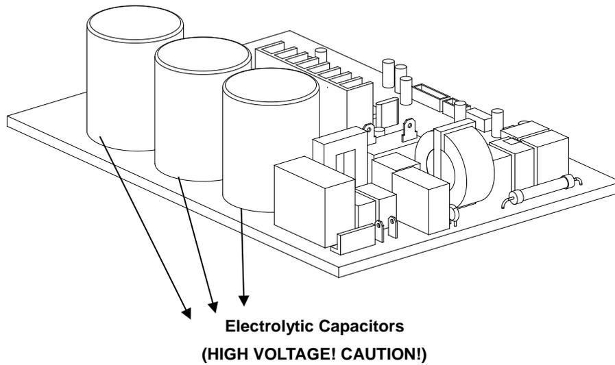
For other models, please connect discharge resistance (approx.100Ω 40W) or soldering iron (plug) between +, - terminals of the electrolytic capacitor on the contrary side of the outdoor PCB.
