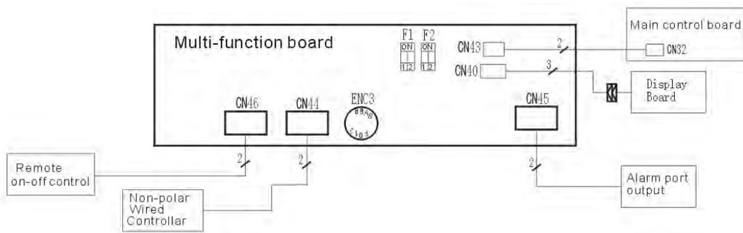
Note: It must use shield cables to connect with Non-polar wired controller.
