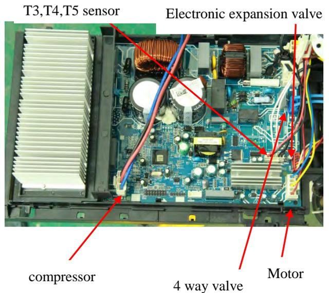
4) Disconnect the connector for fan motor from the electronic control board.
